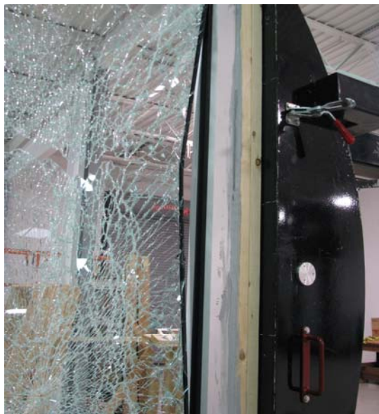
Photo No. 7 Post-test Specimen #1 and #2, Typical Tearing and Pull-out
